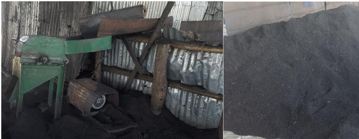
Figure 15 — Crushing hammer mill and sorted charcoal dust
